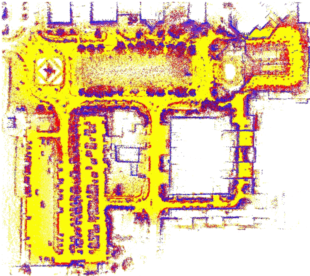
Fig. 8. Top view of the resulting MLS map with a cell size of 50cm x 50cm. The yellow/light gray surface patches are classified as traversable. The area scanned by the robot spans approximately 300 by 250 meters. During the data acquisition, the robot traversed five nested loops with a length of approximately 2,300m.
